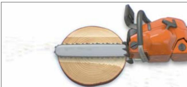
Start by making a bore. Saw through the trunk and complete the hinge width.
