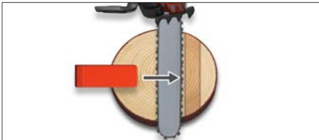
It is very important that the felling cut is sawn parallel to the directional notch to ensure an equal thickness along the length of the hinge.
