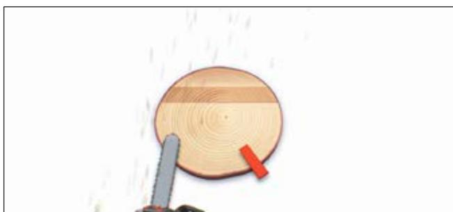
Finally saw off the corner, preferably diagonally down to avoid cutting into the breaking bar / wedge.
