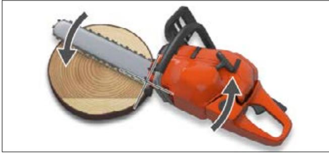
You can also saw from the opposite direction using a pushing chain and apply the upper tip of the bumper spike. However, sawing this way usually becomes more irregular and there is greater engine resistance.
