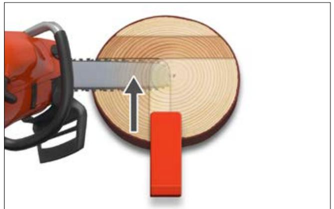
This saw cut can be slightly below the previous cut so that you avoid sawing against the wedge or breaking bar.
