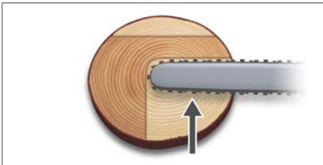
Make the first cut from behind but make sure to save an edge on the opposite side of the tree.
