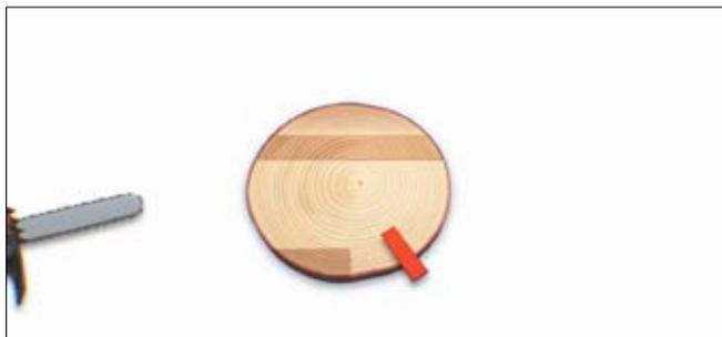
Insert the wedge or breaking bar.
