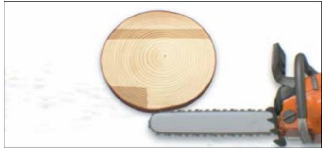
Continue to saw backwards until two-thirds of the trunk is sawn. Pull back the guide bar to create a 5–10 cm wide corner. Then continue sawing until you cut through the tree. All that then remains is a corner of unsawn timber. The corner should have roughly the same total area as the hinge.
