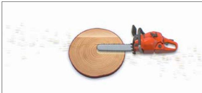
Make a bore cut to about 60 % of the tree diameter.
