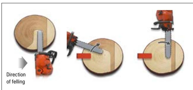
Make a bore as deep as possible. Saw to a suitable hinge thickness parallel to the directional notch. Saw straight back, approximately one guide bar width. Swing the saw around the trunk but avoid sawing into the hinge. Do not forget to pause to insert the wedge or breaking bar. Continue to swing the saw, completing the felling cut and creating a hinge with a uniform thickness and even cut (very important!).
