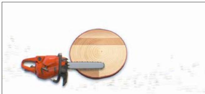
Change your position to the other side of the tree. Make a bore at 60 % of the tree diameter and cut straight backward until you have shaped a suitable corner.
