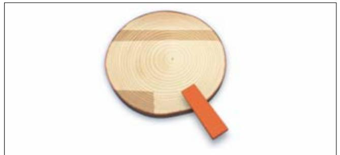
Drive a wedge in the saw cut straight from behind.
