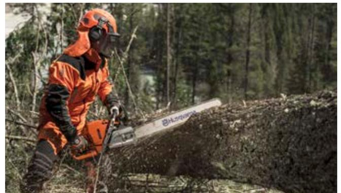
The appropriate length of the guide bar is determined by tree size and to some extent by the user's expertise level. If you are used to handling a chainsaw, you should have access to at least two different guide bar lengths, allowing you to vary the guide bar length with different tree sizes. A shorter guide bar weighs less and is easier to manoeuvre when doing limbing work. The long guide bar is used for larger tree sizes.
